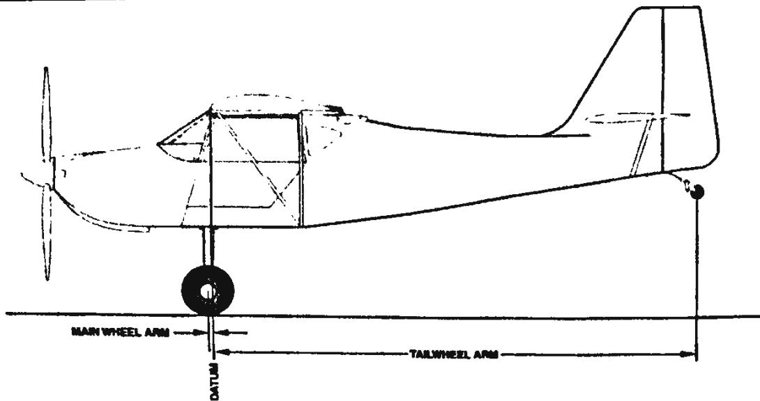
Reference Datum: Inboard leading edge of wing Leveling Means: Level on longitudinal floor tubing below the cabin
